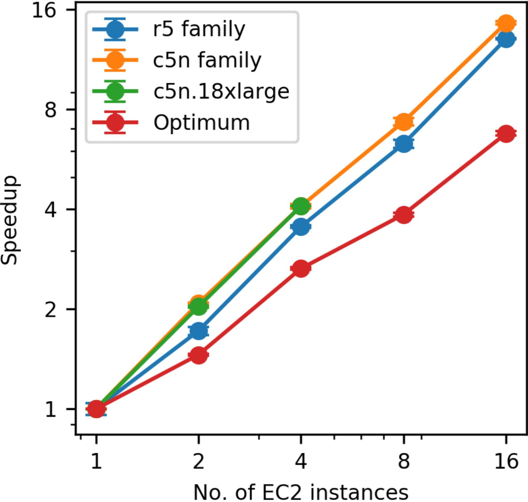
These are best-case scenario experiments: one process/thread per **node** (i.e., the whole bandwidth at full disposal)
