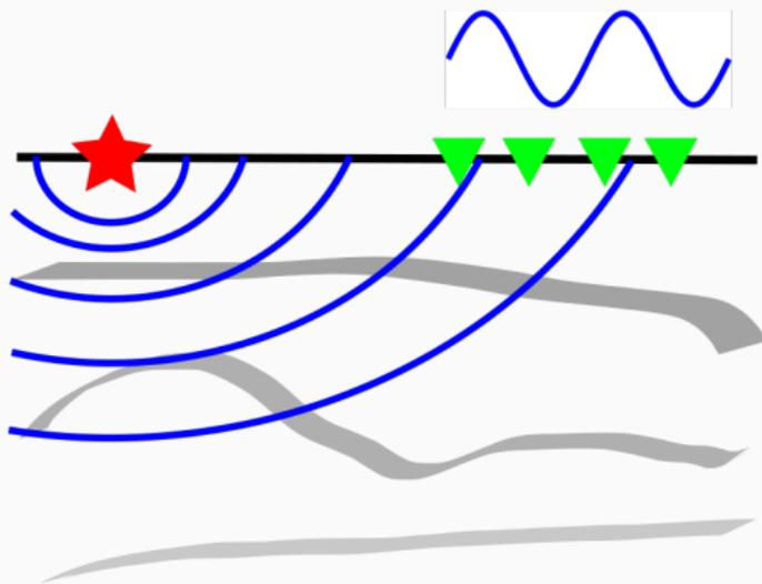
**Figure 2:** Illustration of the forward problem - simulating the received signal for a given structure
