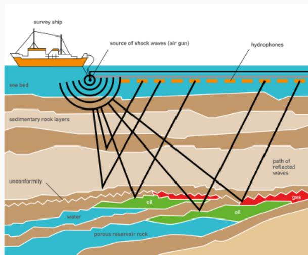
**Figure 1:** Offshore seismic survey
