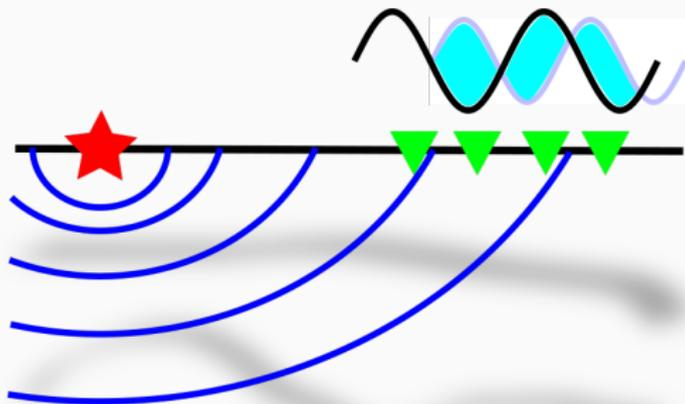
**Figure 3:** Illustration of full waveform inversion - initial guess
