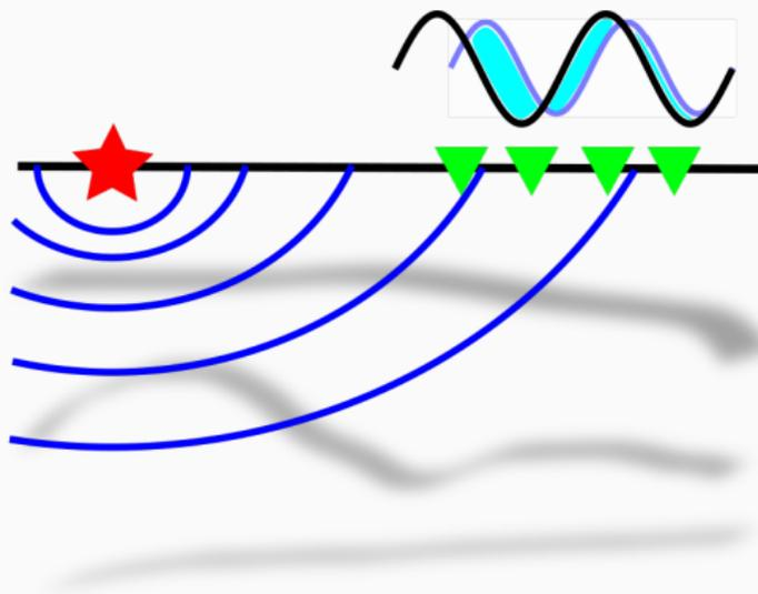
**Figure 4:** Illustration of full waveform inversion - in progress
