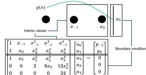
Figure 3: The linear system formed in order to calculate the extrapolation polynomial coefficients, showing where each equation originates. By solving this system for a given set of boundary conditions, polynomial coefficients as functions of interior values and boundary position are obtained. These can then be used to extrapolate the function beyond  $x_b$ , to obtain exterior stencil values.
