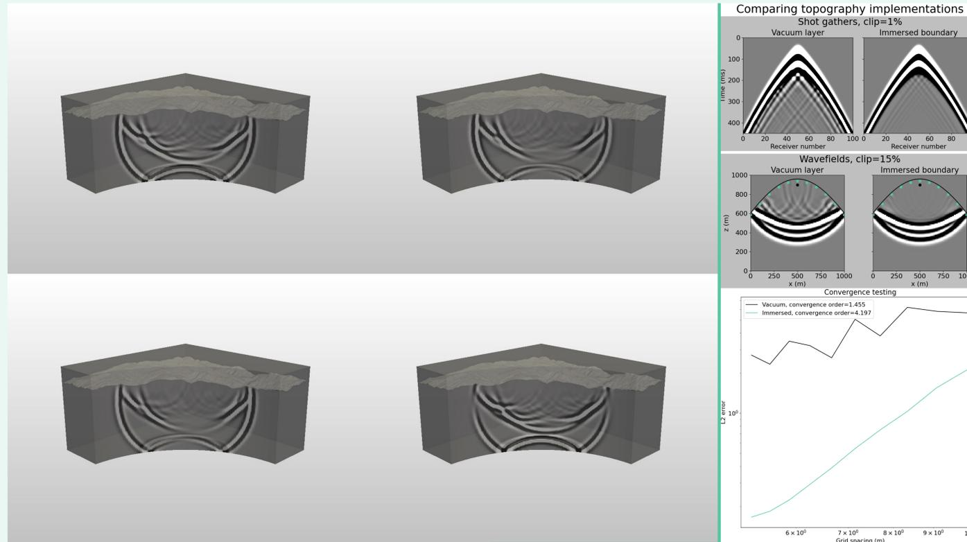
Figure 2: A cutaway render at  $t=4s$  of the wavefields for the topographic scattering model. Counter-clockwise from top left, the renders show pressure, followed by particle velocities in the  $x$ ,  $y$ , and  $z$  directions respectively. The model run demonstrated expected scattering behaviour with only minor distortion of the outgoing wavefront, but numerous chaotic reflections following it.
