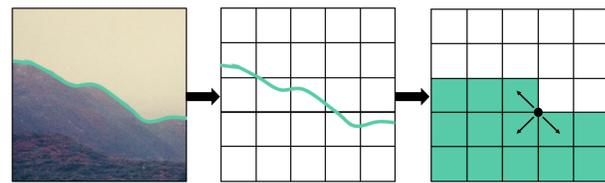
Figure 1: Misrepresentation of topography due to approximation to a regular grid. The smooth topography becomes artificially blocky, producing spurious scatterers, as shown in the third subfigure, where the gentle slope becomes stepped. This staircasing produces both 1st and 2nd-order error<sup>[1]</sup> due to boundary mislocation and material contrast, alongside spurious scattering<sup>[2]</sup>.
